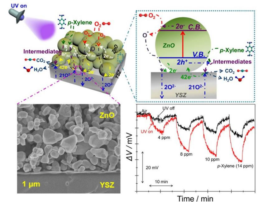
Schema of the light-regulated electrochemical reaction in sensing of volatile compounds.
