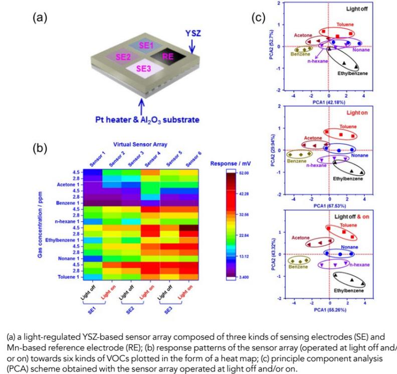
(a) a light-regulated YSZ-based sensor array composed of three kinds of sensing electrodes (SE) and Mn-based reference electrode (RE); (b) response patterns of the sensor array (operated at light off and/or on) towards six kinds of VOCs plotted in the form of a heat map; (c) principle component analysis (PCA) scheme obtained with the sensor array operated at light off and/or on.
